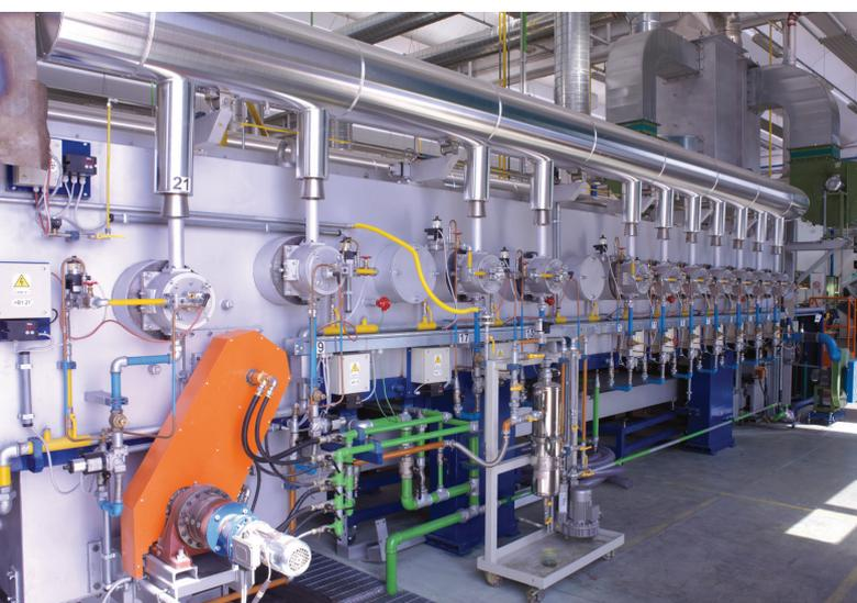
The new heat treatment line can be remotely controlled by a computer system enabling Mecavit to manage, recover and reuse the heat produced, contributing to energy savings.
